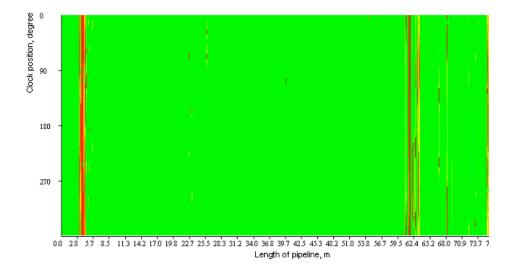
The second shows how this information can be represented to show the density of anomalies (and therefore defects) in the axial plane and a more quantified representation of the degree of danger (ref y axis). Note that F (y axis) is an integral index of the degree
